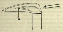
FIG. 2.—REDUCING FLAME, SHOWING POSITION OF BLOWPIPE AND POINT OF REDUCTION.
